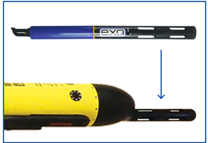
Figure 4. An EXO1 sonde (top) and the specially modified EXO1 that is in the nose of the i3XO.
