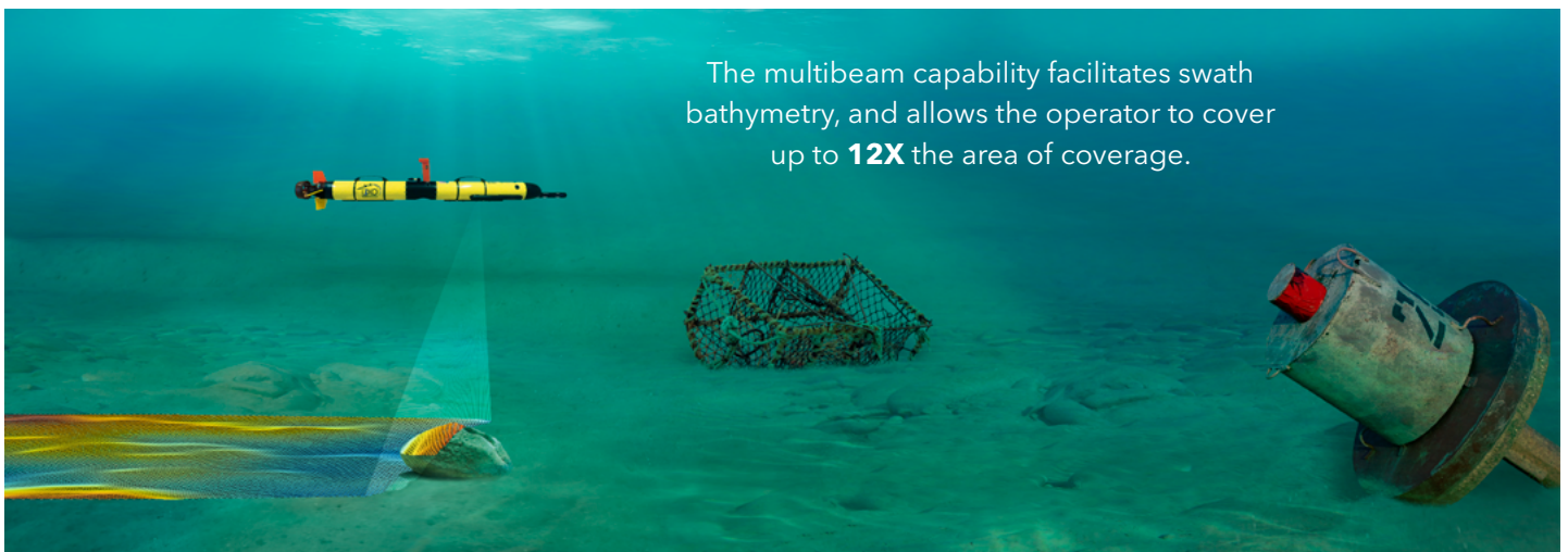
Figure 5. Multibeam side-scan sonar for lake bottom mapping and identification of features.
